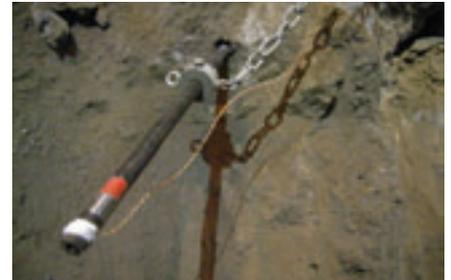
**Above:** An HPCO<sub>2</sub> tube is secured in position using chains, which prevent it recoiling upon activation. **Below:** Examples of the compacted ash deposits that can be removed using KRR HPCO<sub>2</sub>.
