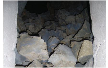
Above: An HPCO 2 tube is secured in position using chains, which prevent it recoiling upon activation. Below: Examples of the compacted ash deposits that can be removed using KRR HPCO 2 .
