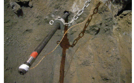
Above: An HPCO 2 tube is secured in position using chains, which prevent it recoiling upon activation. Below: Examples of the compacted ash deposits that can be removed using KRR HPCO 2 .
